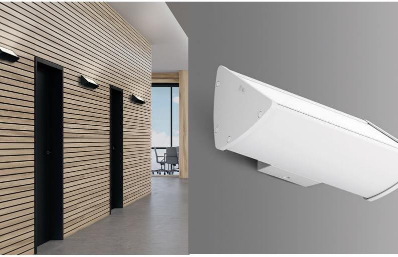
Wall lamp for direct or indirect light depending on the installation. Structure in extruded aluminium alloy 6060/T6. Die-cast aluminium details. Polyester powder coating and phosphate treatment to increase corrosion resistance. Diffuser made of opal polycarbonate, specific for Led, which
